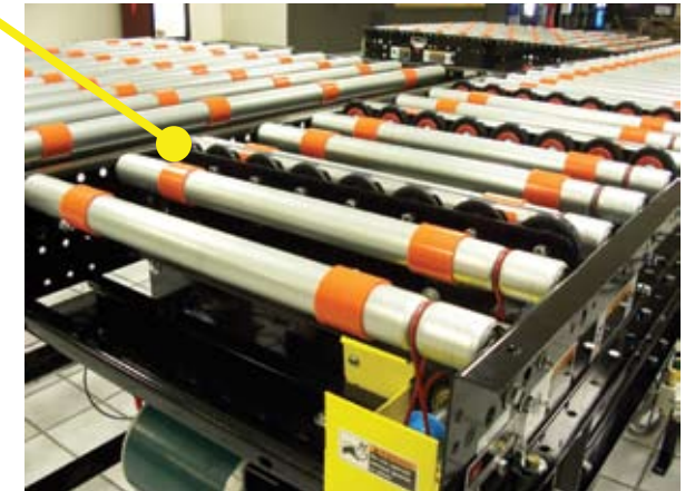
3 Strand Round Belt Transfer makes transition from loading/unloading conveyor to main line smooth and keeps glass from hanging up on rollers.
